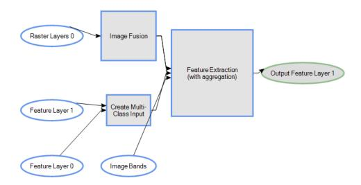
Figure 4. Structure of an AFE file.
